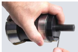
Lock stopper housing in position
